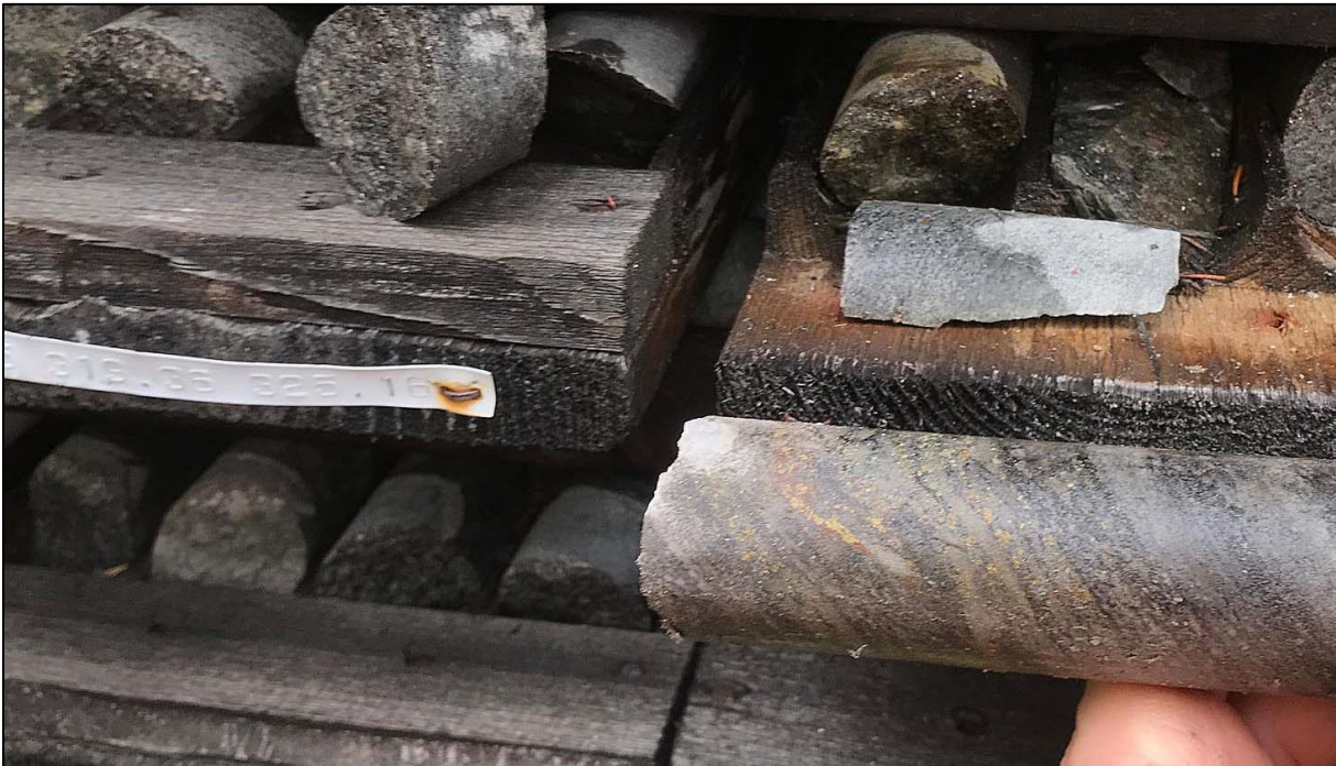
Figure 5. Historical unsampled drill core samples stacked from 2007-2008 drilling at Relf Lake Zone showing unweathered brown ferroan sphalerite-pyrite±chalcopyrite lenses hosted by a quartz-feldspar-biotite±garnet schist 'matrix' with banded 'volcanoclastic' texture.
