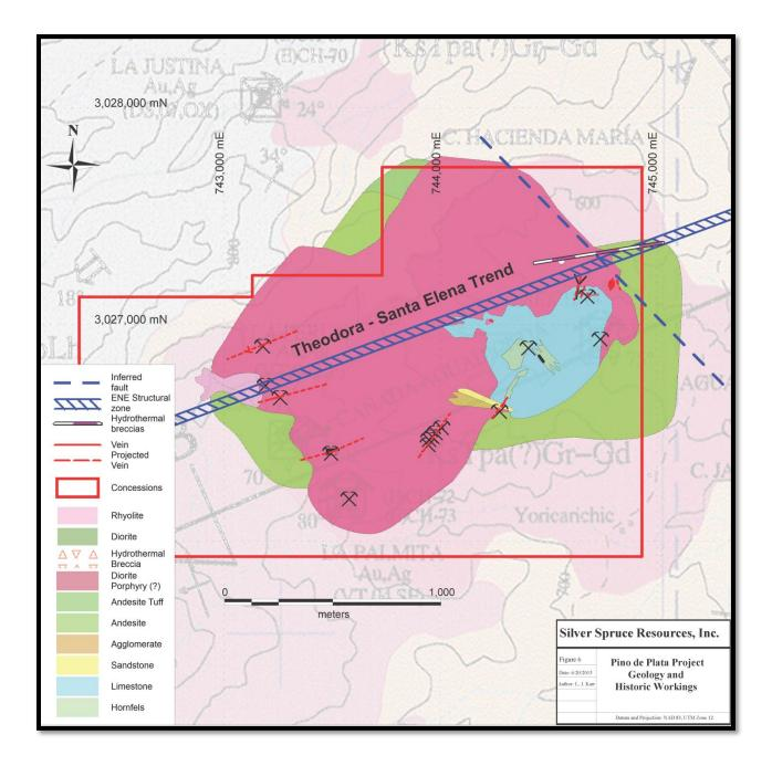
Figure 6. Geologic map of the Pino de Plata Project. Mapping by LJK, May 2015. Geology on underlying base map from SGM Carta Geologico-Minera Chinipas G12-B38. Note that the post-mineral intrusive diorite (different from the mineralizing diorite porphyry) occurs in only two small areas and is not visible at this scale. Note that the perimeter of the drafted lithology portrays the approximate limits of field investigation and not an actual geologic contact.
