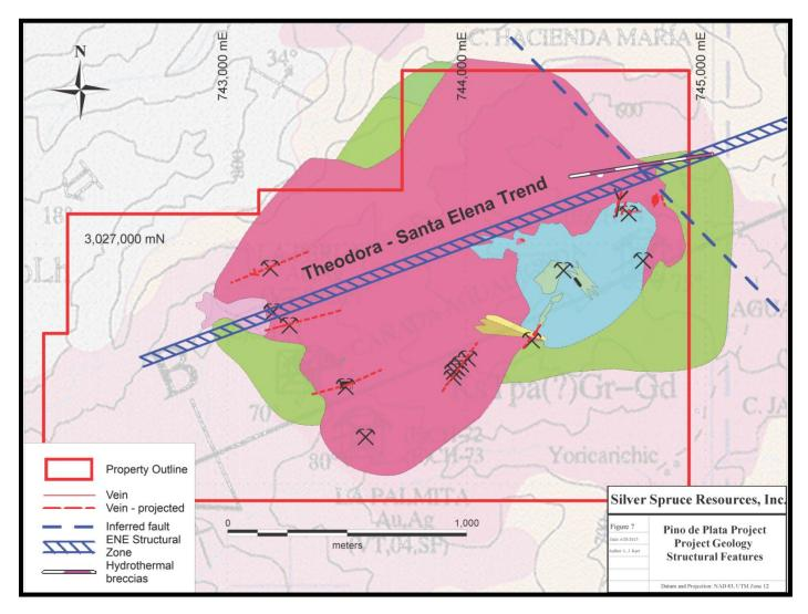
Figure 7. Geologic map of the Pino de Plata Project with inferred fault on east side of property and veins. Veins in the Theodora, Sierpe I and La Perla mines are exaggerated to illustrate their strike. Mapping and interpretation by LJK, May 2015.
