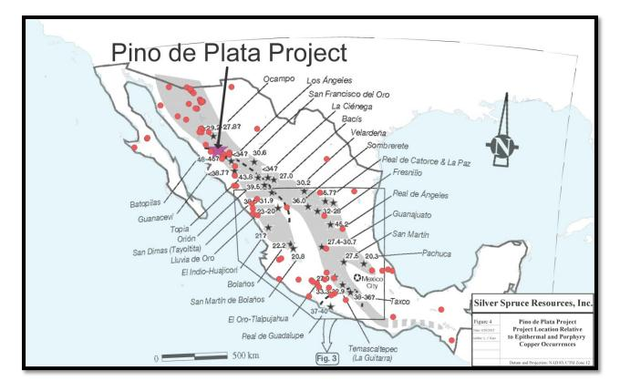
Figure 4. Location of porphyry copper deposits and prospects (red dots) after USGS Porphyry Copper Assessment of Mexico (Hammarstrom, et al, 2010) overlain on figure 2 from Camprubi, et al, 2003; showing ages of select epithermal Au-Ag deposits.
